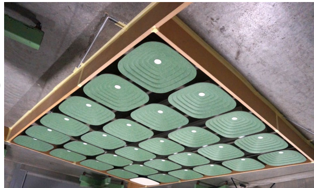
Specimen as tested (image inverted to depict ceiling installation)
